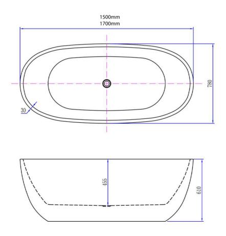
The information contained on this page was correct at date of issue. Fitting dimensions are provided as a guide only. Some variation may occur due to manufacturing tolerances.
